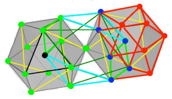
Like the icosa case, in the cubo case there is a central (black) vertex surrounded by 12 (green) cubo-configured vertices and a second layer (blue) forming an intermediate (distorted) cuboctahedron and a third layer (red) forming an outer (more regular) cuboctahedron.
