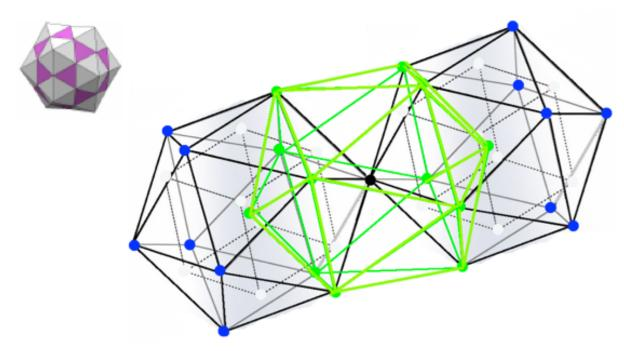
It is a configuration of 2 TSC fusion icosahedra sharing the central vertex with the remaining 55 - (26-1) = 30 vertices in 3 10-vertex bands
