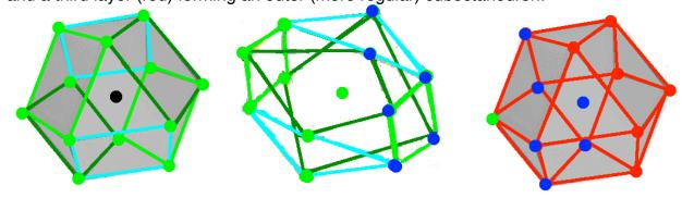
In the cubo case, there are also 12 outer TSC Jitterbug cuboctahedra plus a single central TSC Jitterbug cuboctahedron, so Jitterbug transformation of the entire 147-atom Pd cluster works consistently with individual JItterbug transformations of the 13 TSC icosahedra and TSC Jitterbug cuboctahedra.
