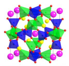
It shows that of the 24 vertices of the sodalite cage, 12 are Aluminum and 12 are Silicon so each Zeolite Cavity has  $10 \times 12 = 120$  Aluminum atoms.
