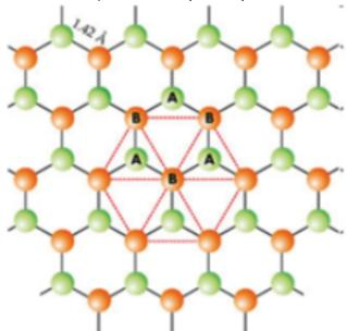
The honeycomb lattice of graphene ... is not a Bravais lattice. Instead, it can be viewed as bipartite lattice composed of two interpenetrating triangular sublattices ... the single-particle electron states are ... two classes, called sigma and pi.
