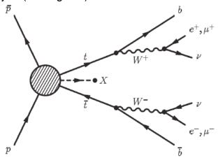
Figure 6.1: Schematic representation of  $t\overline{t}$  production and decay in the dilepton channels.
