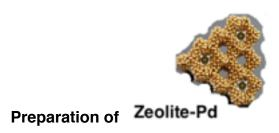
Sodium Zeolite Y has unit cell size about 2.5 nanometers which corresponds to the edge-length per cavity of its overall octahedral structure.
