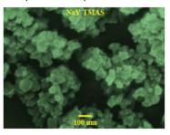
and each unit cell with 1 Cavity is 2.5 nanometers in diameter so an octahedral Zeolite Y Crystal with diameter 35 nanometers would have an edge length 35 / sqrt(2) = 25 nm = 10 cells and the octahedron would have 19 square layers:
