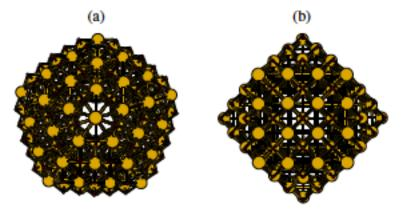
Figure 1. Palladium clusters fully loaded with hydrogen.
