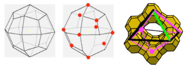
In the center image, the 10 red dots correspond to the 10 sodalite cages. In the right image, magenta is used for hidden lines and for the 2 hidden sodalite cages and
